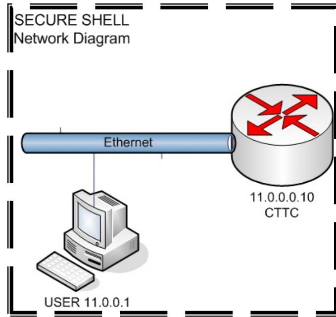
User IP 11.0.0.1 and Connect to 11.0.0.10 fastEthernet0/1 On Router
