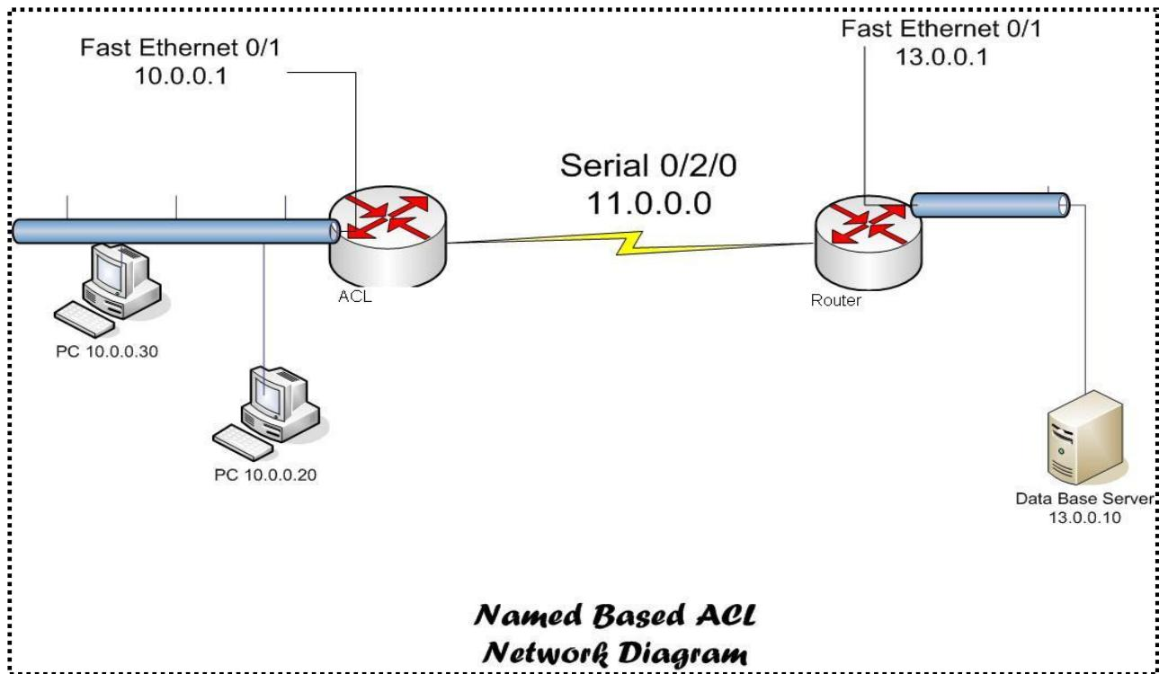
The task on this Lab is to configure a Named Based ACL
